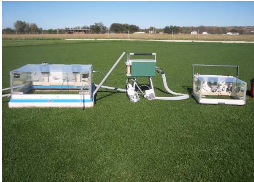
Figure 1. Large chambers cover surface areas of 7.23 \times 10^{-1} \text{ m}^2 (large chamber at left, Murphy, 2007) and 2.4 \times 10^{-1} \text{ m}^2 (mid-sized chamber at right). The small chamber attached to a Licor 6400 (center) covers only 7.09 \times 10^{-3} \text{ m}^2 .
