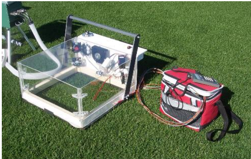
Figure 2. Large chamber fabricated to measure \text{CO}_2 fluxes in turfgrass. The system was connected to and controlled by a datalogger in the red cooler.
